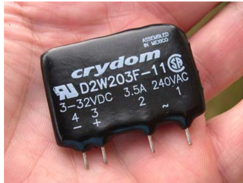
Figure 130.1: A Crydom DW2 Series SSR
